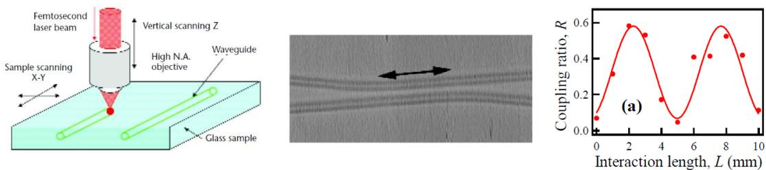
Figure 2- Femtosecond pulsed lasers can be used to write waveguides in fused silica [1].
