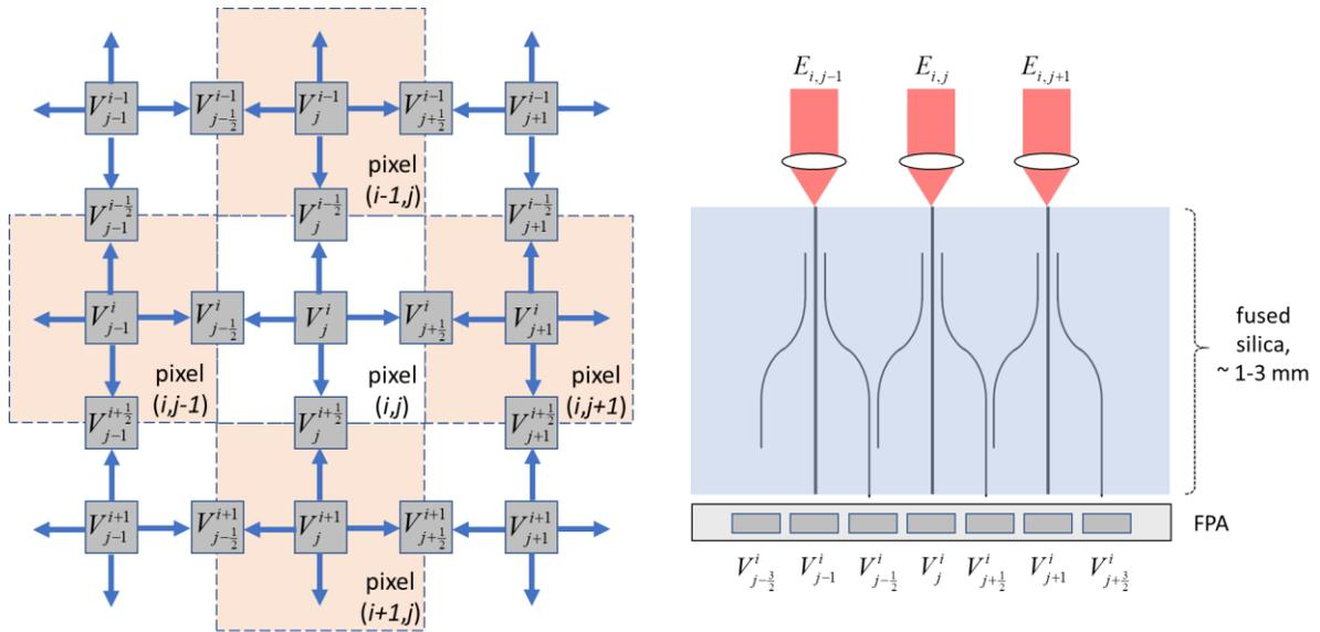
Figure 1 - Diagram of the pixel array connected to the 3D waveguide structure for interferometric coherent sensing on a chip.
